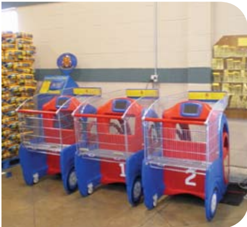
Shopping trolleys recharging via coils embedded in a power mat.
